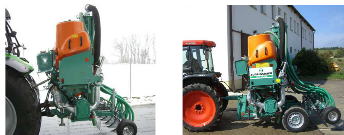
1000 l tank, 12 port distributor. Quick change of applied rate. Different ground applicators
